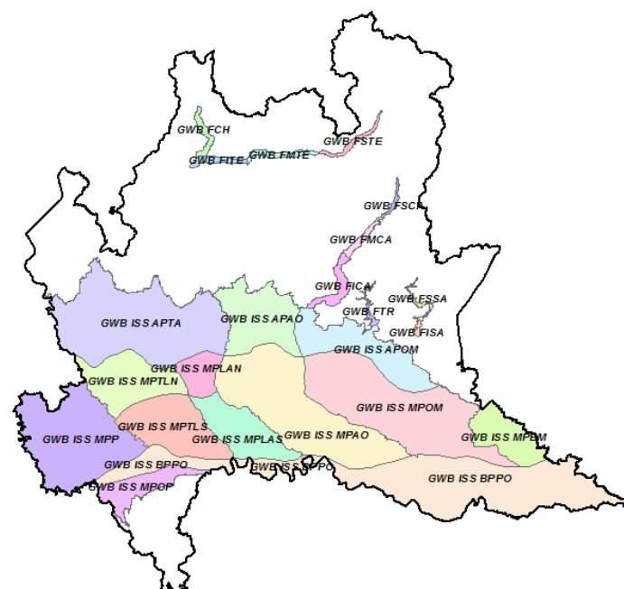
Figure 83: Limits and codes of groundwater bodies (GWB) defined in Lombardy, under the Water Framework Directive; the map shows the superficial groundwater bodies (GWB ISS) and the local GWB in the main alpine valley (GWB F).
